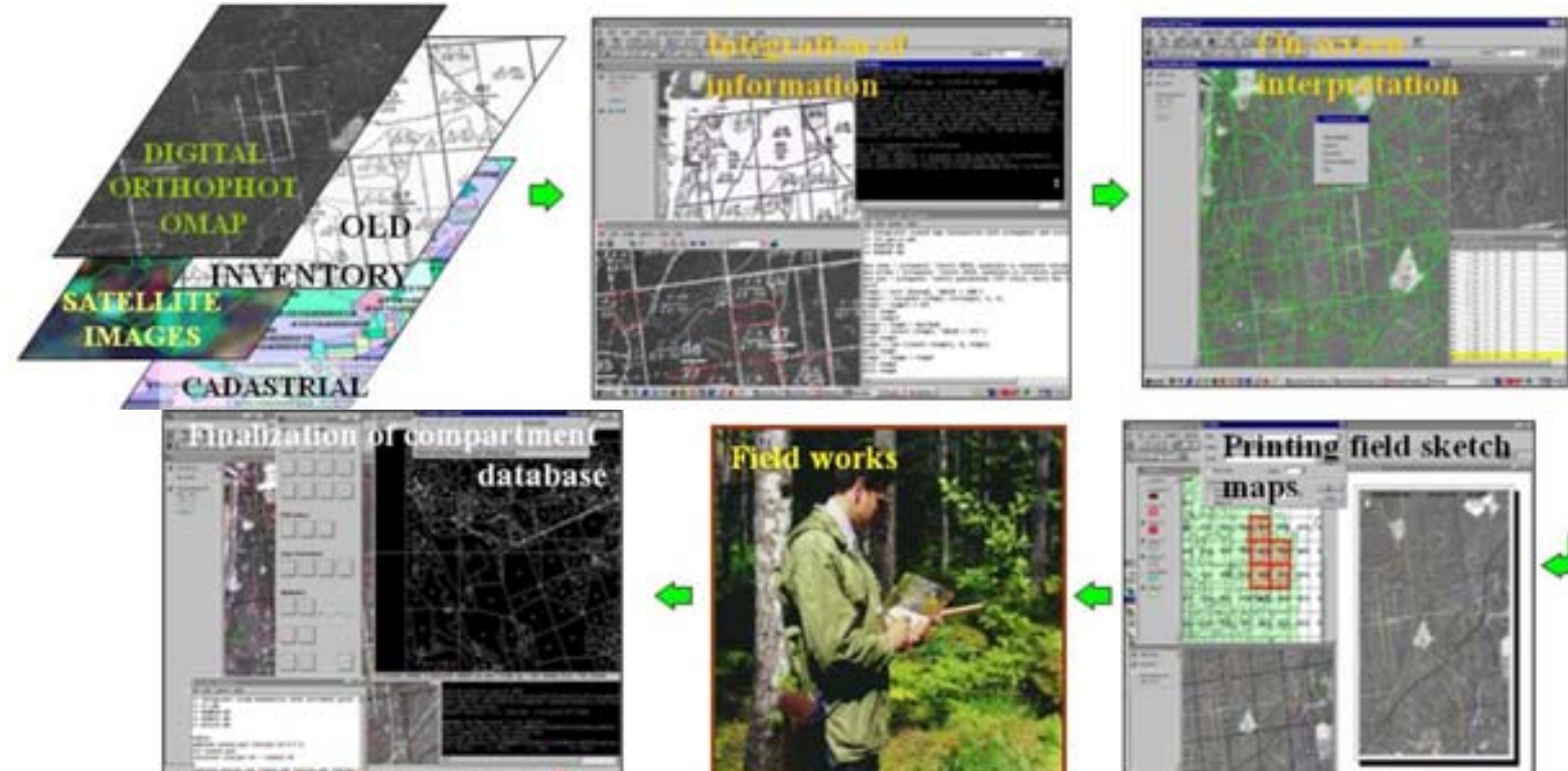
Fig. 3. Main stages of a technology to develop forest resource GIS database in Forest Inventory and Management Planning Institute
